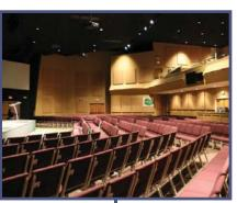
In a place of Worship, sometimes you can hear the sermon, but you cannot understand much or all of it. This is due to excessive reverberation and/or a poor sound system. More frequently it is the space that needs correction – not the sound system and no amount of investment in the sound system can correct the characteristics of the space. They are separate and distinct but must work together.
